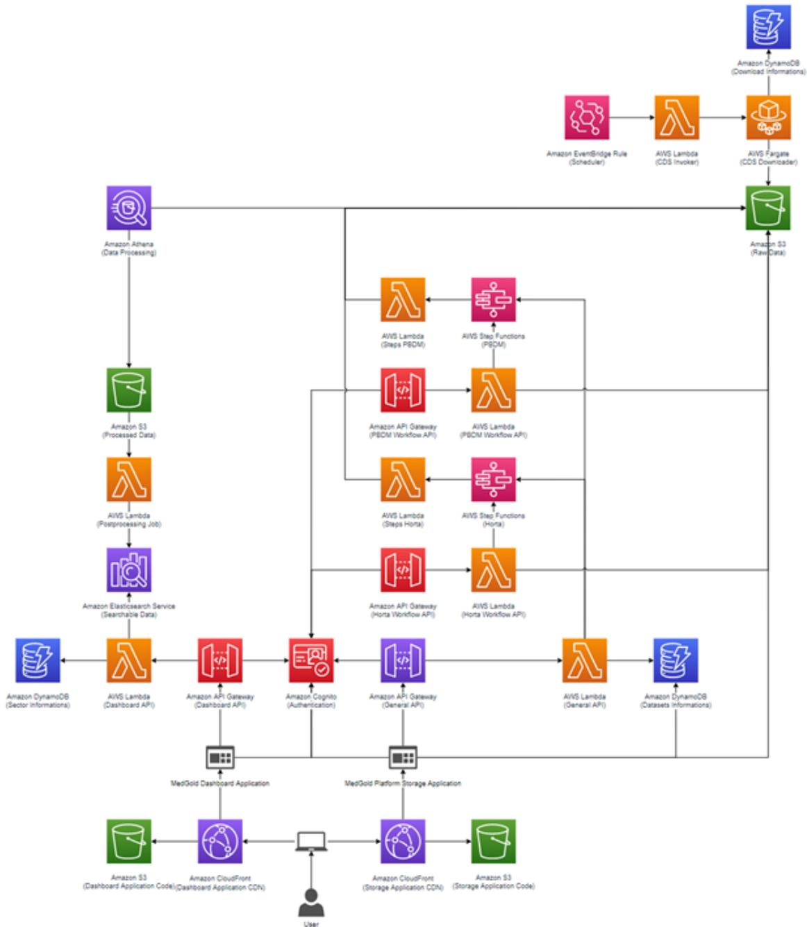
The data processing workflow of the ICT platform typically begins on top of the diagram: a scheduled AWS Lambda Function periodically runs a task on Amazon Fargate (on ECS – Elastic Container Service) to download CDS-C3S data to a local storage location: an S3 Bucket; here the data is processed and forwarded as input of the subsequent step of the workflow. Moreover, information and metadata related to each downloaded file is stored on an Amazon DynamoDB table.
